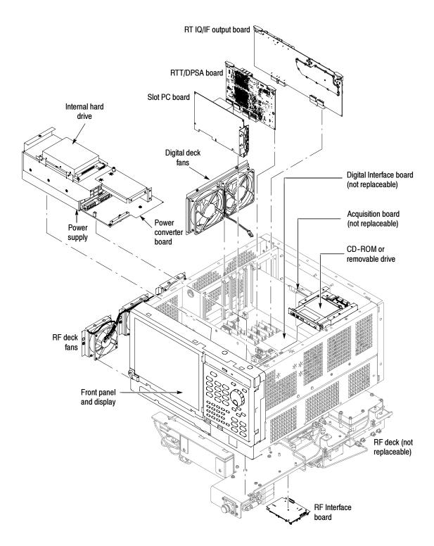
Figure 4-1: Primary customer replaceable module locations
