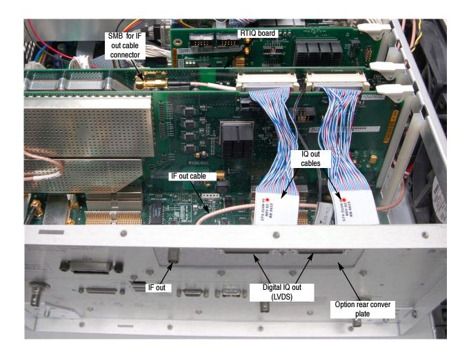
Figure 5-9: Detail of cabling shown in Figure 5-6 (cont.)
