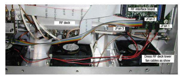
Figure 5-14: Detail of cabling shown in Figure 5-13
