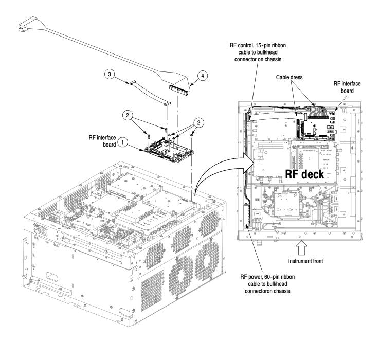
Figure 5-15: RF interface board and cables
