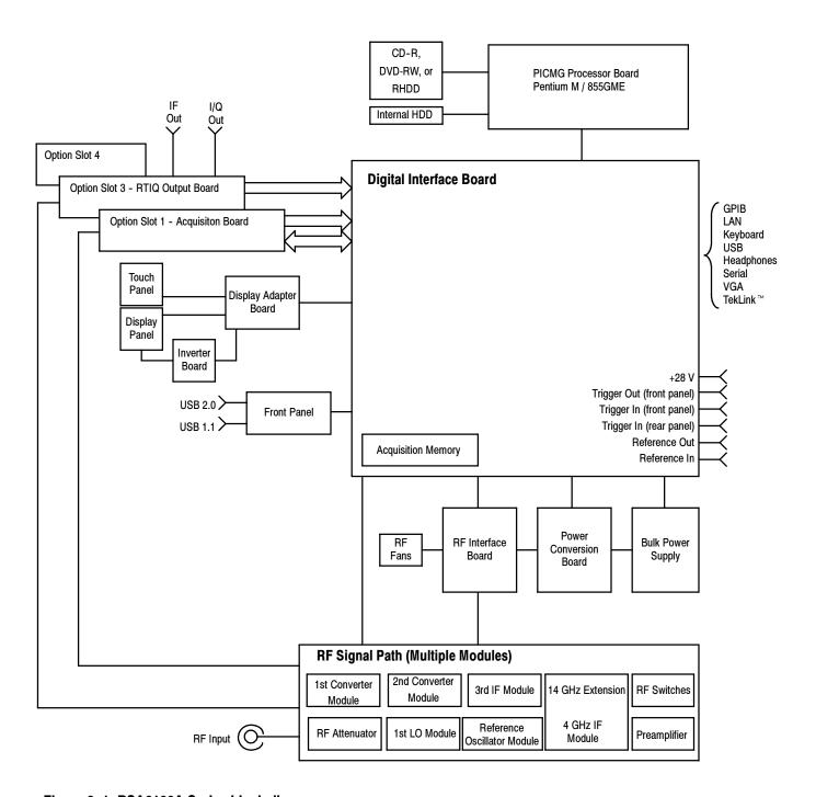
Figure 2-1: RSA6100A Series block diagram
