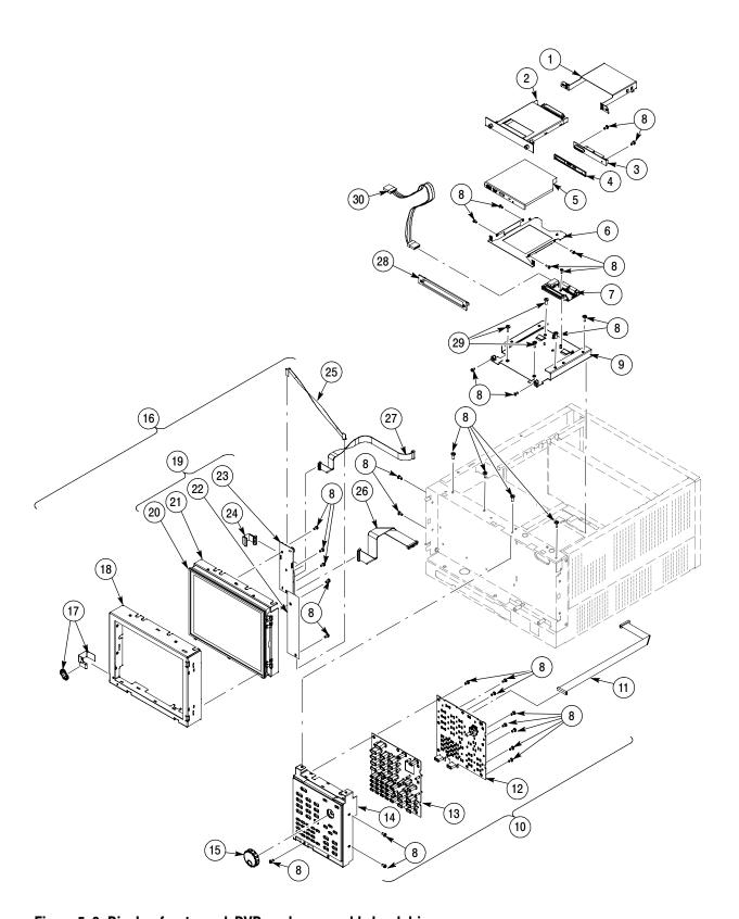
Figure 5-2: Display, front panel, DVD, and removeable hard drive
