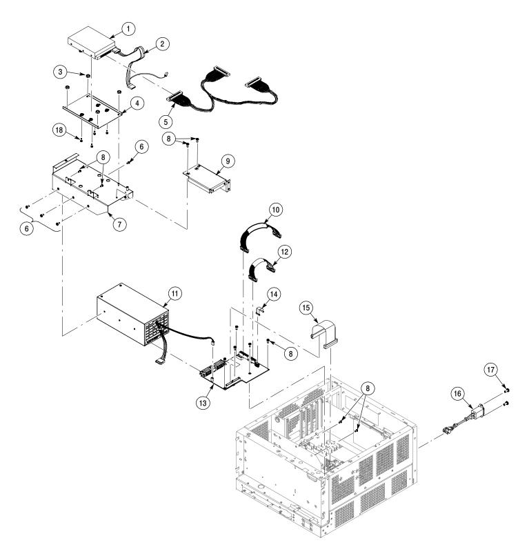
Figure 5-10: Power supply and internal hard drive
