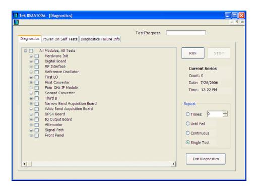
Figure 4-9: Embedded Diagnostics Interface
