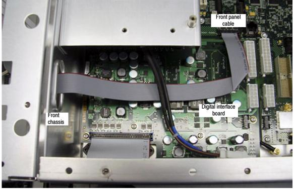
Figure 5-5: Detail 3 of cabling shown in Figure 5-2
