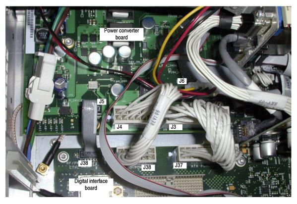
Figure 5-11: Detail 1 of cabling shown in Figure 5-10
