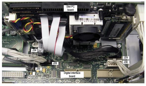
Figure 5-8: Detail 2 of Slot PC Cabling shown in Figure 5-6
